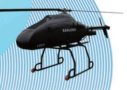
• VE-20 is a small unmanned helicopter designed with high strength airframe and equipped with EFI engine. VE-20 takes off and lands with very less regards to takeoff and landing fields while as a UAS it owns autonomous mission capability. The highlighted liquid cooling EFI engine makes VE-20 fit well in adverse environment. VE-20 is also equipped with advanced terrain follow system to patrol above complex terrain.
